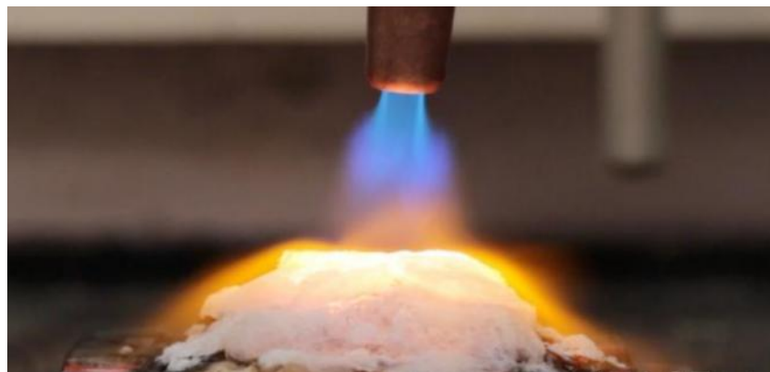
Figure 7: Schematic diagram of the seamless transition of the hydrogel into a strong aerogel shield after heating Source: Advanced Materials
