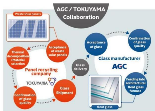
Figure 3: Schematic diagram of recycling process Source: AGC Group
